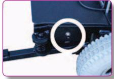
On/Off Switch for Electronic Controls
