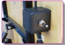
Manual Switch to Move Overboard (Up/Down)
